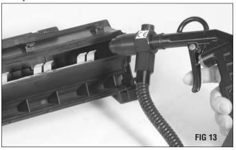
**2.** SCC recommends sealing the cartridge to ensure against toner leakage. For complete sealing instructions refer to SSS™ 453; Phaser® 3400/3450; Samsung® 2150/2550 Adhesive Seal.
