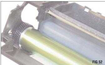
**15.** Push the Drum Axle toward the helical side of the Drum as shown (FIG 53 & 54).. The threaded side of Drum Axle goes on the helical gear side of the Drum.
